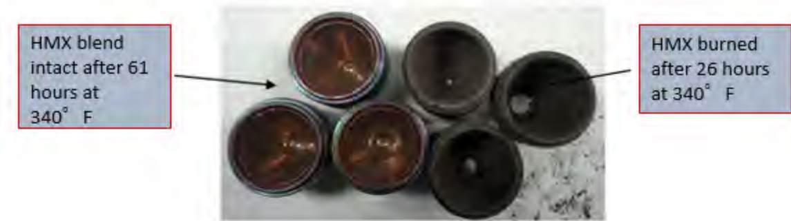
Penetration Comparisons before and after heating at 340F for 61 hours
