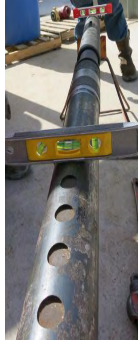
Aligning release tool to first gun module
