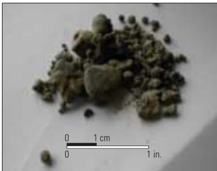
^ Zinc oxide precipitation. Zinc detonation by-products may react with wellbore and formation fluids to form zinc oxide precipitate. The material may precipitate within the formation, perforation tunnels and the wellbore, resulting in an increased reservoir-skin factor and plugged perforations. Large nuggets, such as those shown here, can plug downhole safety and well-control equipment, posing serious operational risk and remediation problems.
