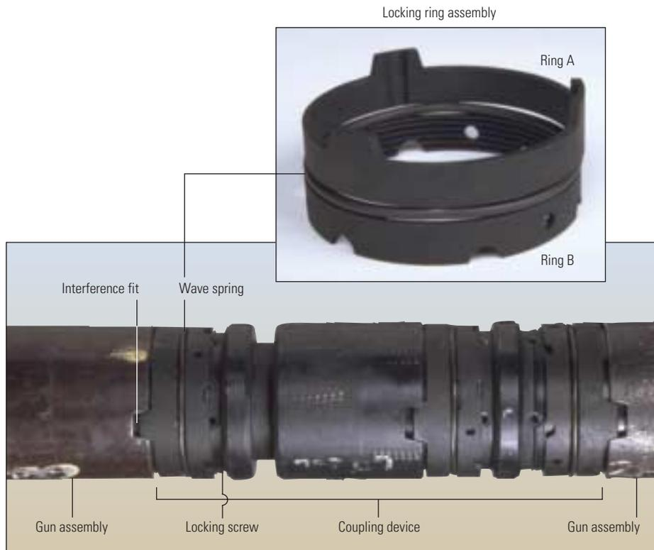
^ Eliminating rotation at connections. Each gun is aligned and locked to the next with an interference-fit notched and keyed coupling device. During assembly, locking Ring A on the coupling device is forced into the female notches in the gun barrel and held in place by a wave spring and shoulder Ring B. The design eliminates play, or rotation, between gun sections. Achieving cumulative alignment errors of less than 10 minutes of a degree per gun assembly is not uncommon.
