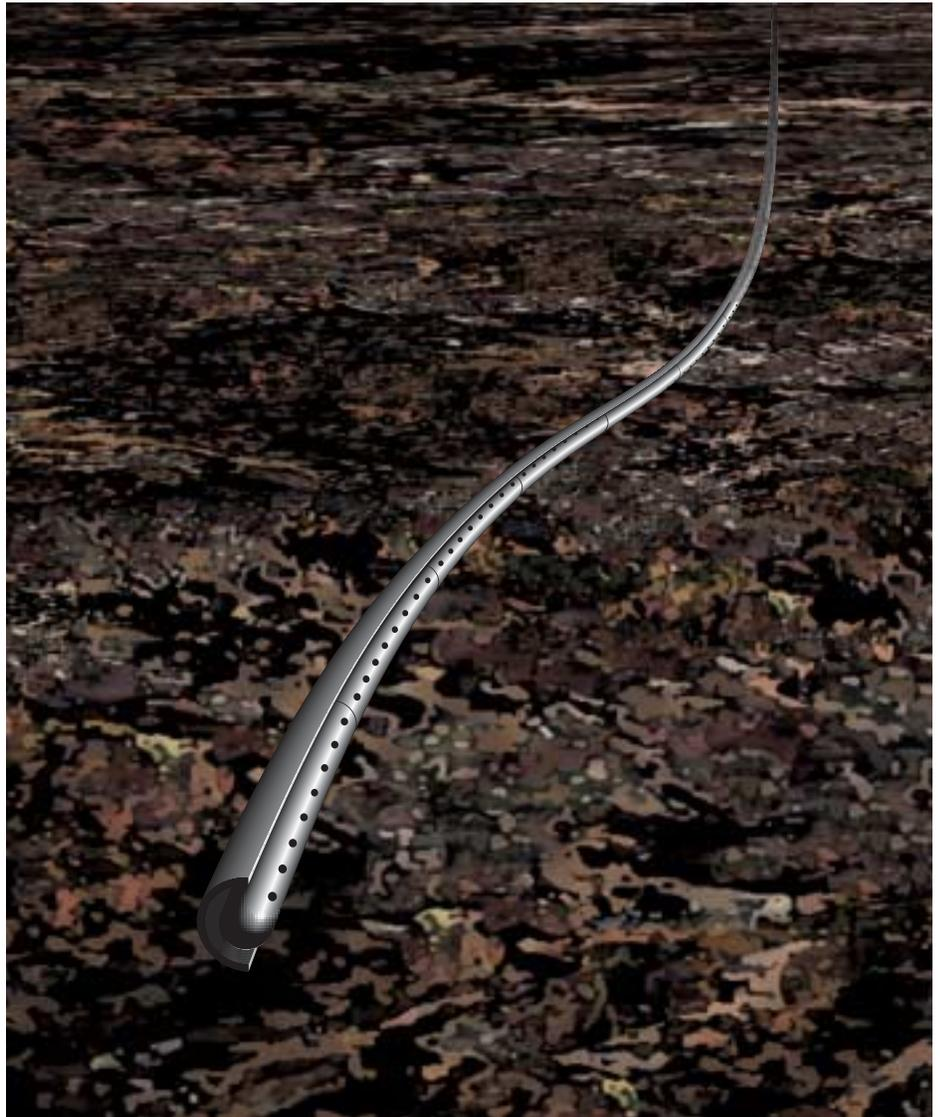
^ Bend-free gun carrier material. With conventional gun carrier materials, rotational torque generated by running the perforating string into the wellbore will rotate perforating guns away from their intended orientation. New bend-free carrier designs, advances in material science and tight manufacturing tolerances allow OrientXact gun strings to bend through wellbore deviations without causing gun misalignment.
