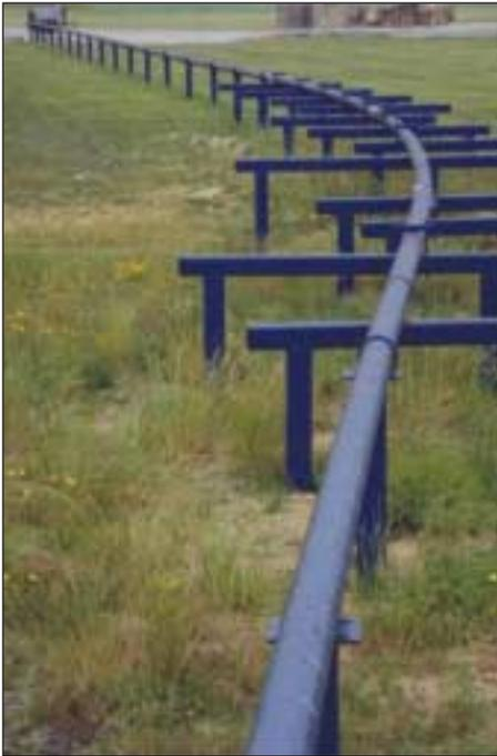
^ Making the bend in performance testing. At the Schlumberger Reservoir Completions Technology Center in Rosharon, Texas, USA, the OrientXact system was tested at bends ranging from 5°/100 ft [5°/30 m] to 10°/100 ft [10°/30 m]. Wireline-conveyed gyroscopes confirmed orientation variance at 6° or less through the bend sections, indicating that the OrientXact swivel and gun carrier designs would perform as required by Hydro in field applications with severe doglegs.
