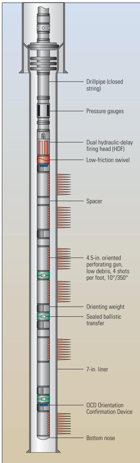
^ Design of the OrientXact tool tubing-conveyed oriented perforating system. The OrientXact design directs all perforations in a vertical direction with 10°/350° gun phasing. Pressure gauges may be used to record pressure changes during discharge. One or more low-friction swivels support the gun string. Two OCD Orientation Confirmation Device units are located at opposite ends of each swivel-supported section. The need for orienting weights is determined based on rotational torque requirements.
