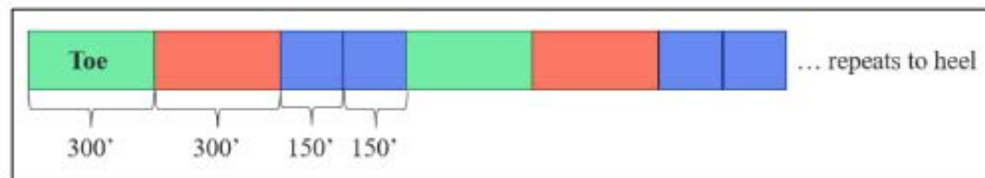
Figure 1—Simple design summary alternating stage architecture every 300'.
