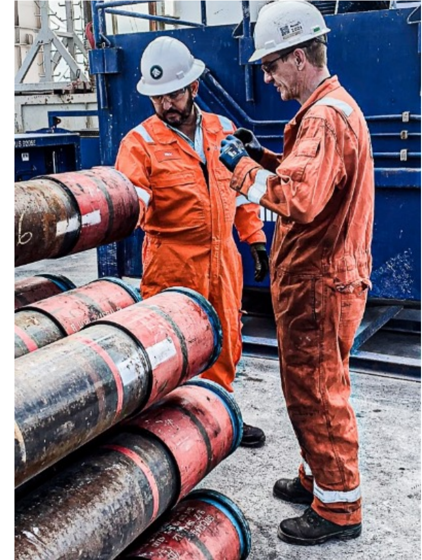
Ref: Personnel inspecting GRE casing during the Rig Visit
