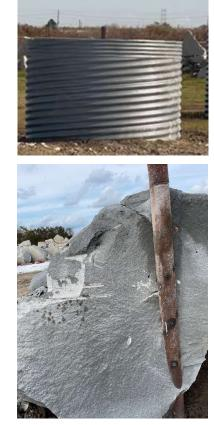
API 19B S1 cement target: OD=72-in, >=28 days Gun size: 3.12-in. Casing: 5.5-in, 20# P110
