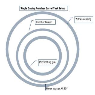
Barrel test setup:
