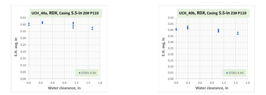
• UCH\_40 tested for 2 casing weight, the results EH and stdev are almost the same, though casing wall 0.05" difference.
