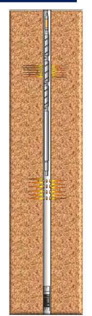
firing head Gun#4 firing head Gun#3 firing head Gun#2 firing head Gun#1
