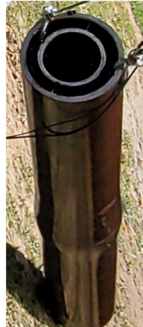
7 5/8" O.D. x 6.625" I.D., 39#, Q-125 11 3/4" O.D. x 10.282" I.D., 82.69# Q-125
