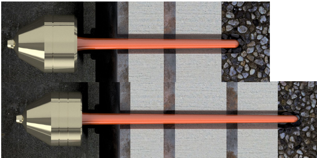
Figure 16: Multiple casing, formation reaching, shaped charges illustration. Adapted from DynaEnergetics media library.
