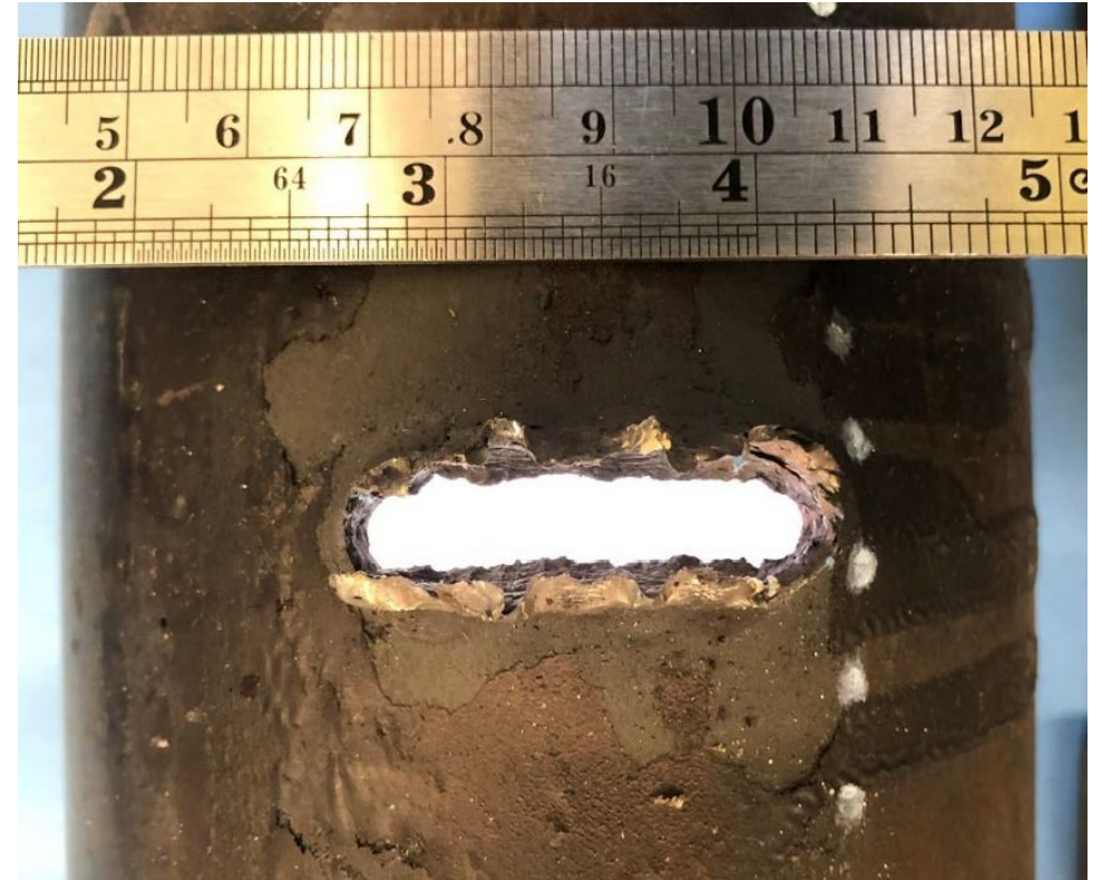
Figure 13: Slot opened in a 4-1/2 inch tubing. Adapted from DynaEnergetics media library.
