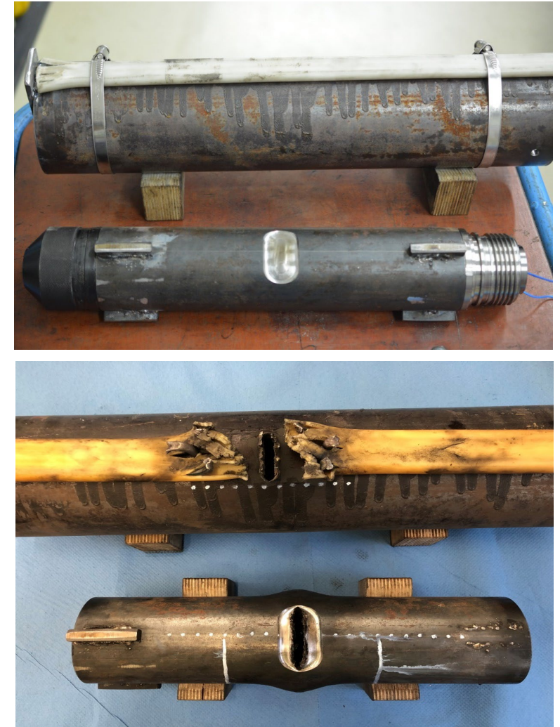
Figure 11: Pressure vessel test setup, for cutting capabilities confirmation. Adapted from DynaEnergetics media library.
