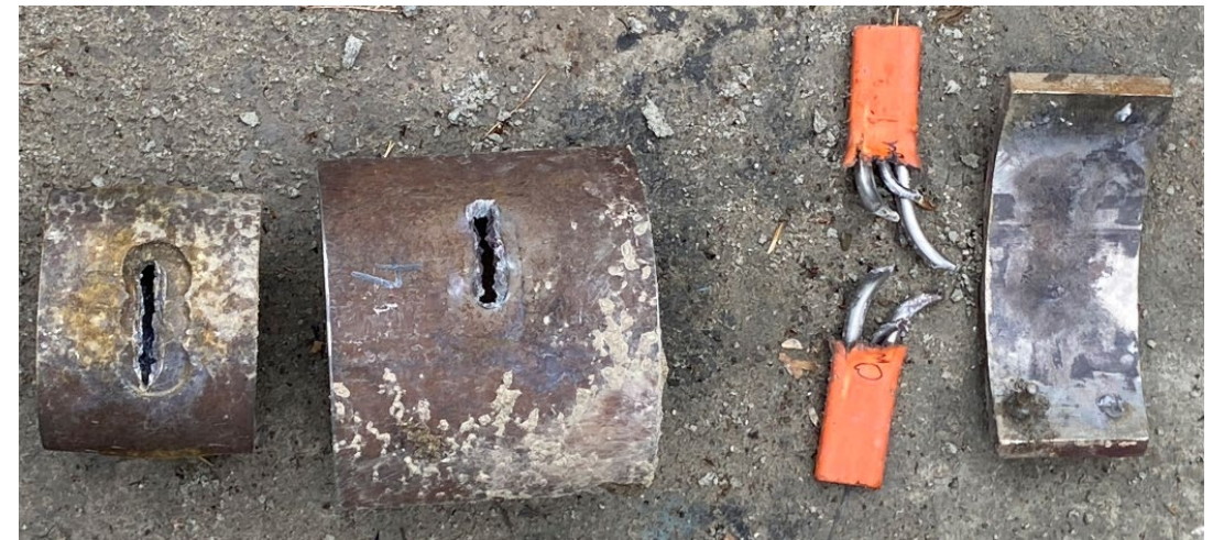
Figure 10: Coupon test setup, for cutting capabilities confirmation. Adapted from DynaEnergetics media library.
