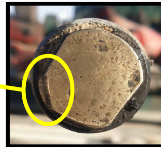
Deep Mark of Drop Bar at the 1.5" ID Crossover. X/O was at depth 3327m (which was above BPV)
