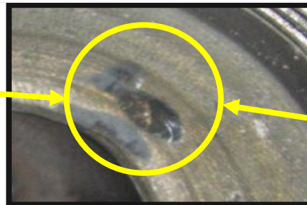
Deep Mark of Drop Bar at the 1.5" ID Crossover. X/O was at depth 3327m (which was above BPV)
