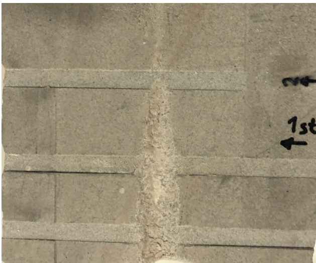
Fig. 10: Three scratch test profiles (bottom, middle and top) were measured across the tunnel with approximately 2" distance between them on the second half of the rock shown in Fig. 2.
