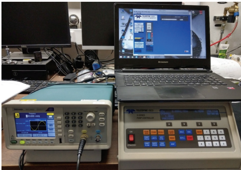
Fig. 6: The control unit of the syringe pump was connected to a PC, which recorded the measured flow rates and pressures. A function generator on the left was attached to the input of the control unit to regulate the flow rate.
