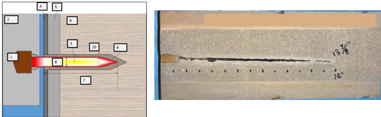
Figure 1a. Schematics of the perforating geometry: 1. Perforating Charge, 2. Perforating Gun, 3. Perforation jet, 4. Casing, 5. Cement, 6. Reservoir rock, 7. Perforation tunnel length, 8. Entrance Hole Diameter, 9. Crushed zone, 10. Crushed Zone Thickness. Figure 1b Image of a perforated core, the tunnel and the damaged zone are clearly visible (Grove, et al. 2012)
