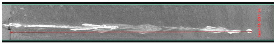
CT scan image after perforating. Notice no cavity was formed near the perforation entrance on the left and even after the hot water displaced the majority of the crude oil coating the sand grains.
