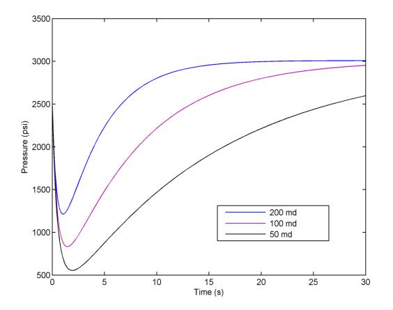
Plot shows an example where the model can be quickly used to understand the influence of core permeability on the dynamics of the pressure curve.
