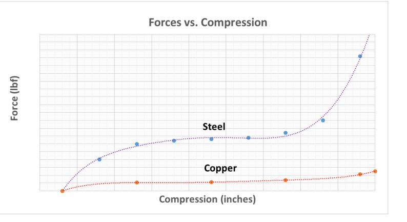
Steel crushable element can absorb more detonation energy through the deformation of coiled tube due to its higher yield strength
