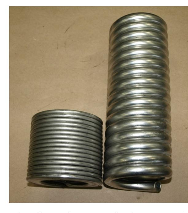
Shock isolation device is designed by a passive shock isolation mechanism with a shock absorber, which is usually a crushable or spring-dashpot element to dissipate the detrimental energy. It is simple and effective for the application in a specific frequency band and energy level, etc. In this work, we present a new design of crushable shock absorber with adaptive
