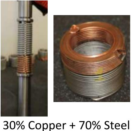
Test Results of Crushable Elements
