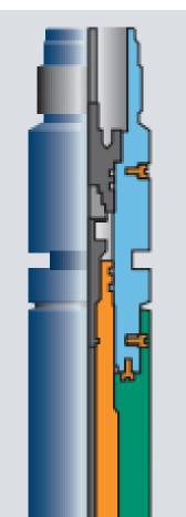
During a perforating job, the detonation and its induced pressure wave in fluids produces large magnitude stress wave in the gun string. It may damage the delicate electronics, as well as, weak mechanical components. Tremendous shock mitigation efforts, such as design of shock isolation devices, optimization of gun string layout, and numerical modeling, have been investigat-
