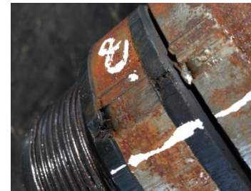
Damaged Seal Assembly from perforating debris
