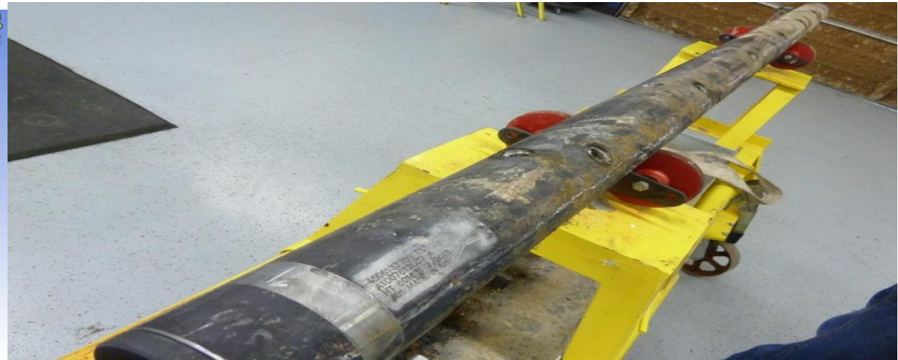
Gun body after ballistic survival shot test
