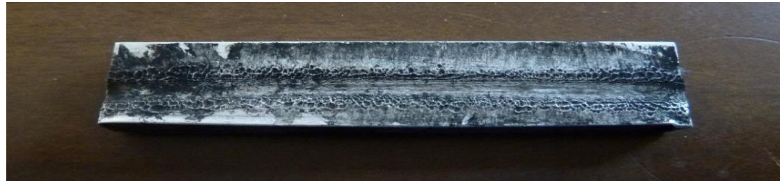
Witness plate from test above, showing high-order detonation of the detonating cord
