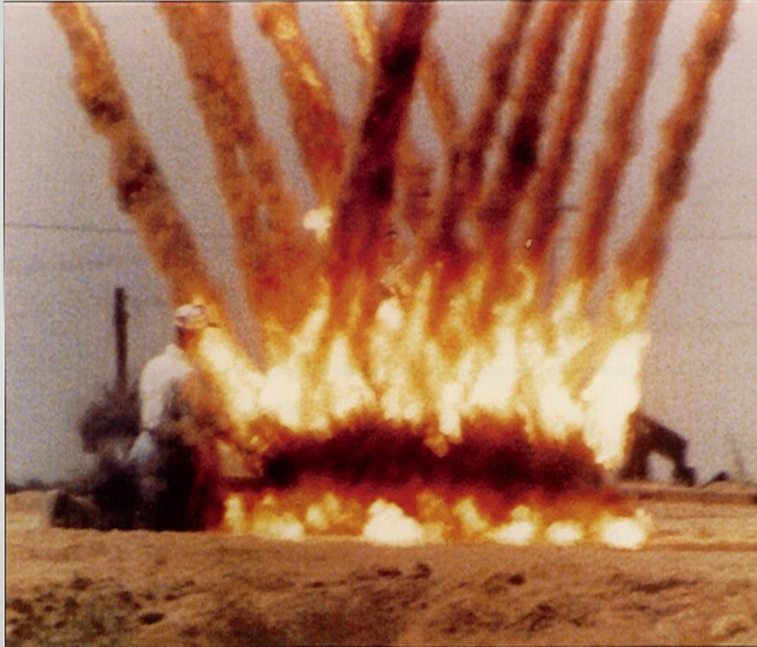
Figure 1-2. The tremendous power of an oilwell perforator demonstrated by a perforating gun detonated at the surface. The figure at left is a mannequin.
