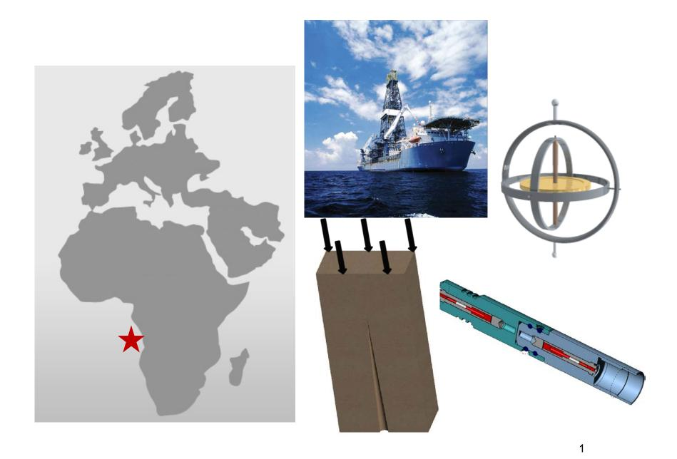
On Deep-water field in particular was trying to use a previous generation of orientation for sand control. These systems and many still used in the industry today allow the casing, friction and well bore debris to interfere with the orientation of the guns. In order to make sure the charges were oriented towards the max stress plan a wireline gyroscope would be run in to verify orientation.
