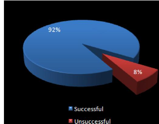
OTC paper identifies in the study that 8 percent of oriented perforating jobs ended in sub optimization which means higher risk of sand production. The majority of these are associated with systems that rely on orientation devices that can be influenced by contact with the casing.
